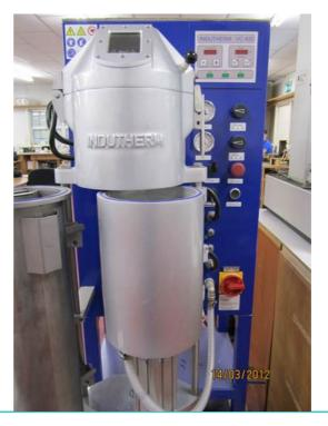
Linn High Term High frequency induction furnace: Titancast 700 mP Vacuum Useful for centrifugal micro casting of titanium, and other alloys, by using the lost was casting process
