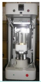
Tribometer Plint TE67-HT (pin-onplate and pin-on disc high temperature machine) Friction and wear tests at macro scale up to 600°C
