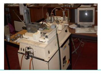
Micro-abrasion test machine, Plint TE66
