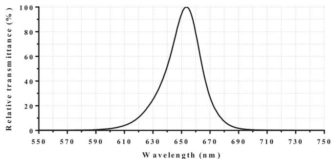
Fig. 2. Relative emission spectrum of LED WP7113SURC/E.
