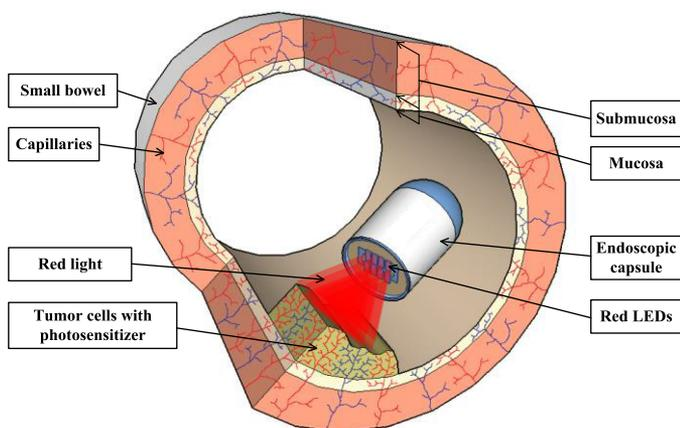
Fig. 1. Illustration of PDT integrated in the endoscopic capsule.
