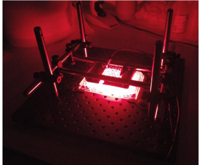
Fig. 4. *In vitro* light treatment of one 96-well plate, in the dark, with the light source and structure presented in Fig. 3.
