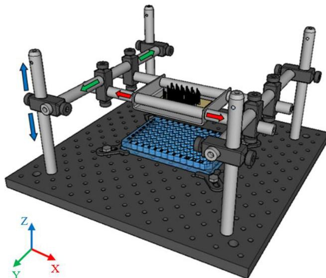
Fig. 3. Structure for supporting and placing the light source above of culture cell plate.
