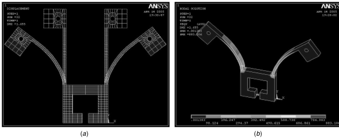
**Figure 11.** Finite element analysis (FEA) of the flexure joints of the asymmetric gripper: deformed and undeformed structure (a) and enlarged view (b).
