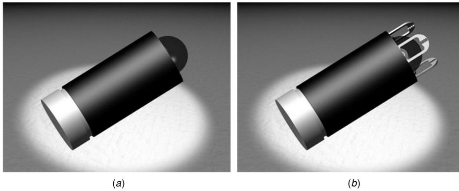
**Figure 1.** Basic concept of a clamping capsule before (a) and after gripper protrusion (b).
