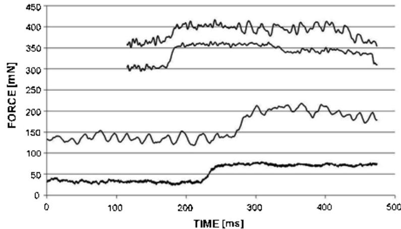
Figure 9. Measurements for the evaluation of the retraction force for the clamping capsule with symmetric gripper.
