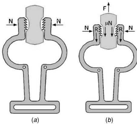
Figure 10. Forces scheme without (a) and with traction (b) for the symmetric gripper.
