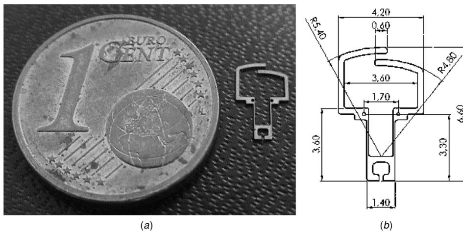
**Figure 12.** Prototype of the asymmetric gripper (a) and dimensions (in mm) (b).
