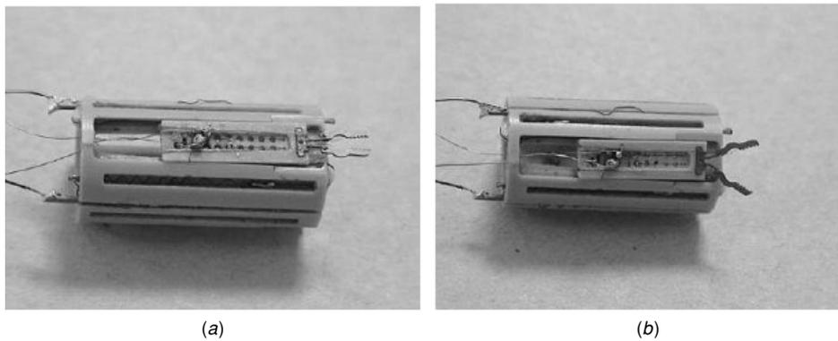
**Figure 6.** Clamping capsule prototype with protruded gripper: closed gripper (a) and open gripper (b).
