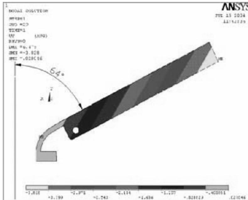
Figure 4. Clamping system FEA (finite element analysis) of the gripper.
