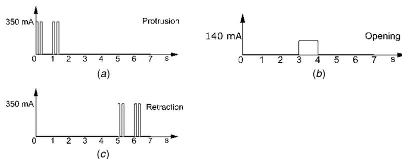
**Figure 7.** Actuation phases: protrusion (a), opening (b) and retraction (c).
