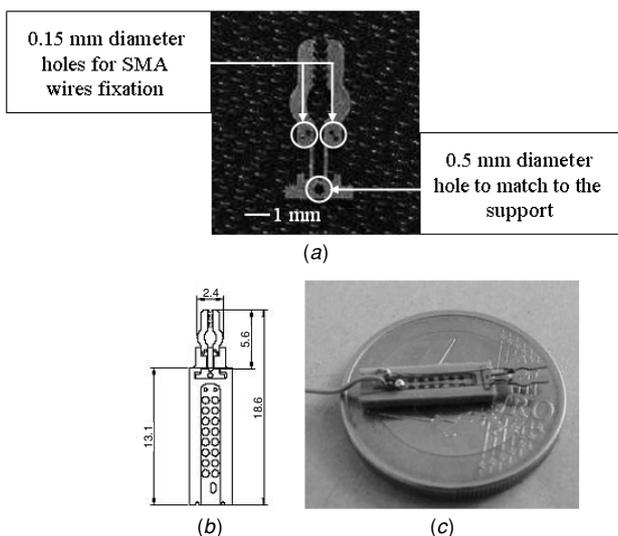
Figure 5. Symmetric gripper: prototype (a), dimensions (in mm) (b) and integration with the support (c).
