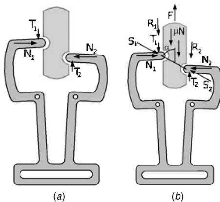
**Figure 17.** Forces scheme without (a) and with traction (b) for the asymmetric gripper.
