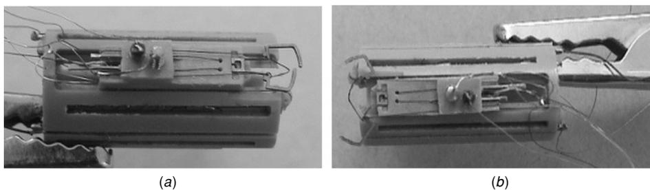
**Figure 13.** Prototype of the clamping capsule with asymmetric gripper: retracted support and closed gripper (a) and protruded support with open gripper (b).
