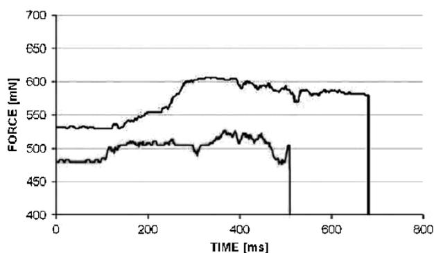
**Figure 14.** Measurements for the evaluation of the retraction force for the clamping capsule with asymmetric gripper.
