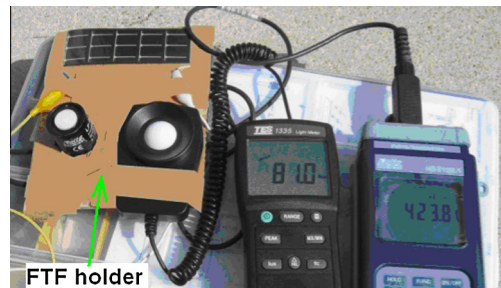
Fig. 5. Photograph showing the optoelectronic measurement setup, where it is possible to observe the luximeter (on left) and the radiometer (on right), whose sensors are positioned in the same plane of the FTF (containing the FTF holder).
