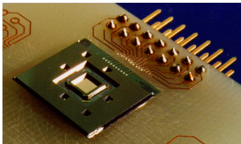
Microspectrometer for UV, visible and IV with digital output and bus interface
